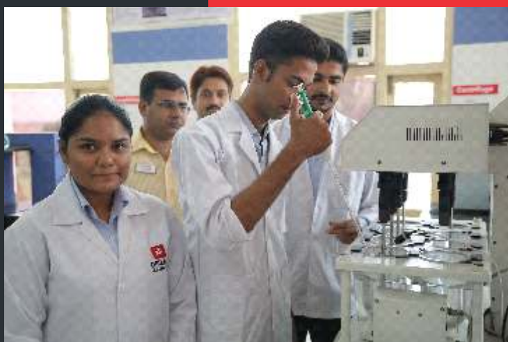
USP 6 BASKET DISSOLUTION TEST EQUIPMENT
