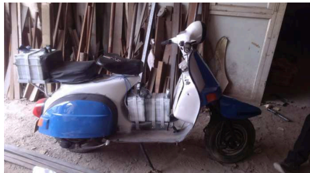
Fig.2 Prototype of Eco-Hybrid scooter
